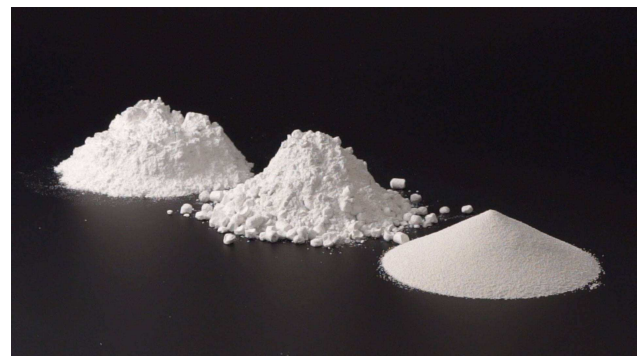
Figure 5: visual aspect of different highly micronized talc grades. From the left: loose powder talc HTP1, compacted talc HTP1c, free flowing talc HTP1s.
